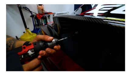
**2.8.** Once the holes are opened up to 3/8", we can now install the rivet nuts. To properly install the rivet nut, you will want to thread the rivet nut onto the tool as shown below, and place the rivet nut into the hole.
