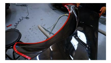
2.13. Place the wing back on the rear hatch and create a small flap by peeling back one end of the red tape backing as shown below. Note: Ensure your mounting bracket holes line up with the rivet nuts properly before final placement of the wing.
