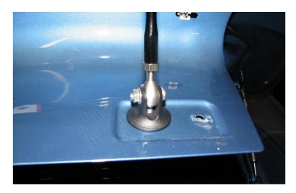
**2.17.** After the bottom clevises are installed, we can install the clevises on the drag wing itself. Do so by threading the M6 x 16mm long low-profile socket head caps screw through the clevis and into the rivet nut as show below. Keep hand tight for right now.
