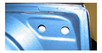
2.7. Once the 4 bolts are removed, carefully and firmly pull the black trim piece away from the trunk. Below is a photo showing what the backside of the trim piece looks like. Note: There are a couple of different mechanisms holding this piece to the trunk apart from the bolts, so it will take some patience and moving the panel in different directions to remove safely.
