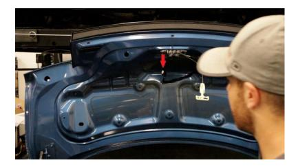
**2.6.** Underneath the black covers that were removed in step 2.4, you should see something like the photo below. Use a 7mm socket to remove these bolts inside the cutouts in the trunk. There are 2 bolts per side that need to be removed.
