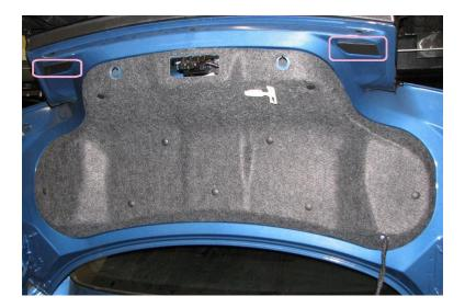
**2.5.** Next, unclip the rear connector for the rear camera.
