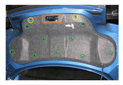
**2.4.** With the sound deadening removed, we need to remove both black covers that are circled in pink below. You can do this by hand or with the help of a flathead screwdriver.
