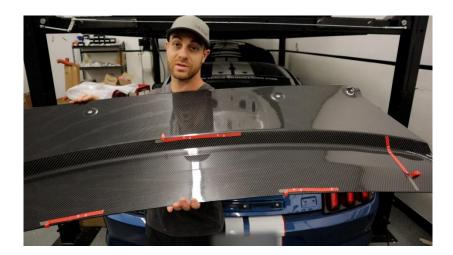
**2.11.** Test fit the wing on the trunk before removing the red backing. The wing should sit into place as it shares the contour of the trunk. Once test fit, peel the red backing away and place the wing on the trunk while massaging it into place.
