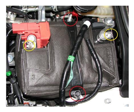
**2.4.** After the battery is removed, we need to install a zip tie or two to hold back a factory hose line from in front of the brake master cylinder. This hose can be seen in the below image.
