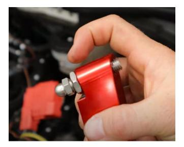
**2.13.** Install the brake master cylinder brace as shown below. Start by hand threading in the 18mm long M4 SHCS and M4 washer then fully tighten to 4 ft-lbs with a 3mm allen wrench. Do the same with the M6 SHCS and M6 12mm Washer using a 5mm allen wrench.
