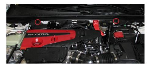
**2.6.** Using scissors, cut out the area in which the rivet nut will be installed and the BMC Brace will sit. We recommend leaving around an inch on either side.
