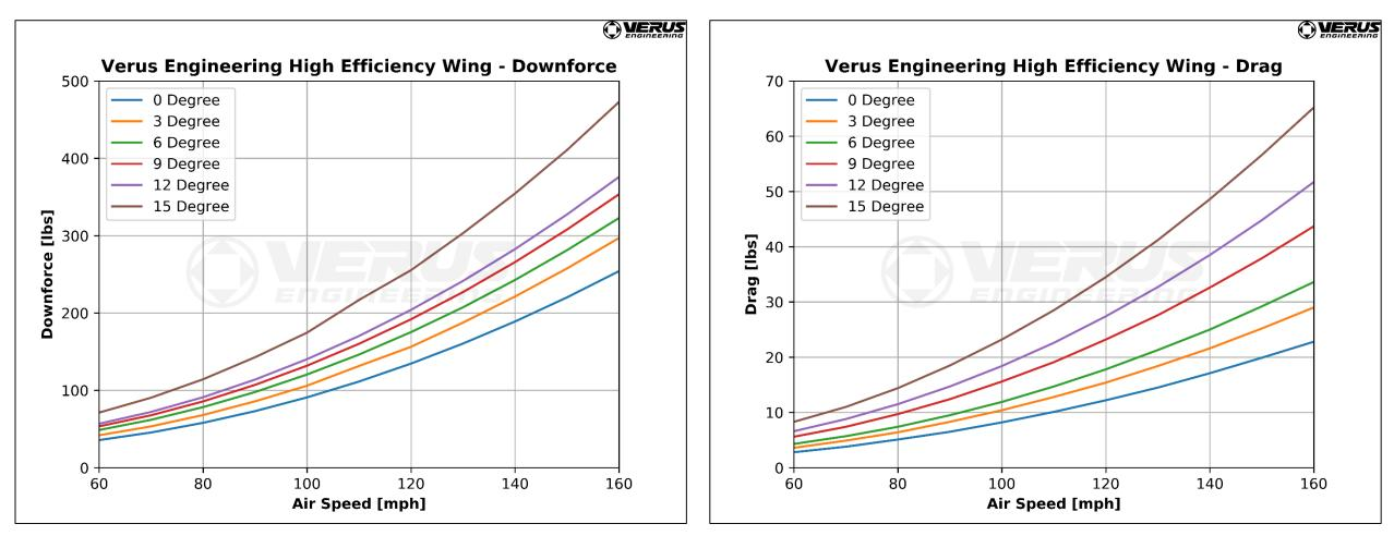
Freestream downforce data on the Verus Engineering High Efficiency Wing which is on the Ventus 2 Package. The data on the car on the previous page is from 6 degrees angle of attack. How the downforce and drag can change based on wing angle change can be calculated using these graphs.
