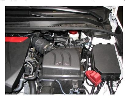
2.3. In order to gain better access to the installation area, we need to remove the top of the air box. Do so by using a Phillips Head Screwdriver or a 10mm socket to loosen the worm drive clamp (yellow circle) and then remove the electrical connectors to the airbox (orange circles). Note: The second photo is not an actual connector, it is just a mounting point for the wiring loom, but it still needs to be removed to remove the top of the airbox.
