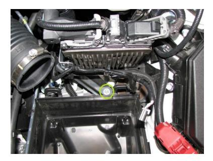
**2.6.** Now that we have more area to work with, remove the 12mm bolt shown below (orange arrow) and the two black stickers (light blue arrows). One sticker is to the left of the bolt and the other is below the bolt. There will be M8 threads behind the stickers we will be utilizing.
