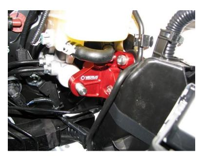
**2.9.** Once the BMC Brace is loosely bolted on the car, we need to place the foot adapter in its location. Do so, by unthreading the brace adjuster until it secures the foot in place against the master cylinder as shown below. Do not fully tighten the brace adjuster or jam nut yet as we will make final adjustments later on. You just want to make sure the foot is held in place for the time being.
