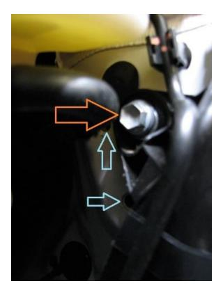
2.7. Before we install the BMC Brace to the car, we need to preinstall the brace adjuster into the BMC Brace as shown below. Ensure the jam nut is installed on the brace adjuster before threading it into the BMC Brace. (Brace adjuster > jam nut > BMC Brace) Do not tighten the jam nut yet as we will need to adjust later on in the install.
