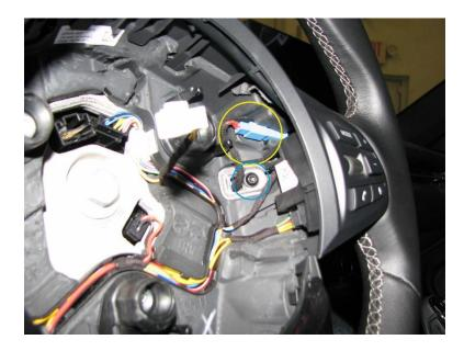
**2.7.** Using a small Phillips screwdriver or a small Allen wrench, push the pin out that is shown below. Fully remove this pin from the assembly and set aside for use with the new paddle shifters.
