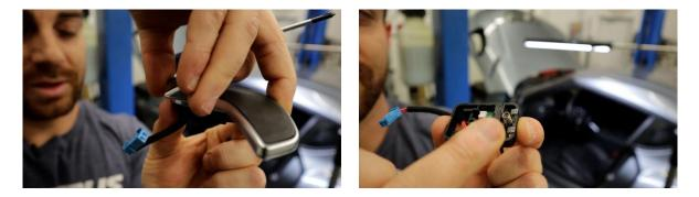
2.9. Now grab the correct side Verus Engineering paddle shifter and reinstall the electronic assembly in reverse order. Fitment will be slightly tighter than OEM, so take your time and be patient during reinstall. Note: Do not forget to reinstall the small black pin that was removed earlier.
