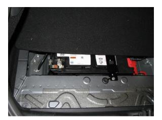
2.3. Once the negative terminal is removed from the battery, the electronic hatch release will no longer be useable for the time being. We advise putting a towel or something similar over the hatch locking mechanism, as shown below, in case the trunk is closed for whatever reason.Note: There is a safety release available, but it will require climbing inside the car to release.
