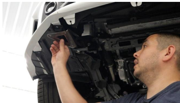
Passenger side bracket installed
