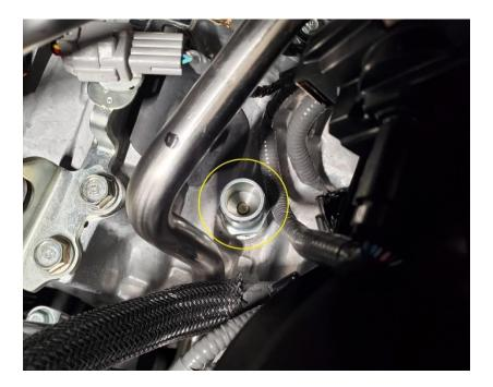
**2.8.** Replace the PCV valve in the engine block with the provided NPT to 1/2" barb fitting. Clean and degrease the threads on both the fitting and the engine block (make sure no debris falls into the engine), and apply thread sealant to the threads on the provided fitting. Tighten the fitting about a 1/4 turn past snug. These are tapered threads, also known as NPT, and should **NOT** be bottomed out.
