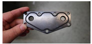
**3.2.** Install the coolant plate between the AOS, and the mounting bracket. Use seven 16mm long M6 BHCS, and torque to 6 ft-lbs. Make sure the o-ring does not become unseated and get pinched.
