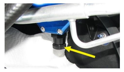
**4.2.** Swap the o-ring over from the knurled plug fitting to the new threaded adapter with the through hole shown below.
