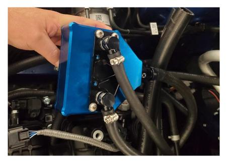
3.6. Bolt the AOS to the fire wall with the two M6 serrated flange nuts just as you would have in2.5. Torque the nuts to 6 ft-lbs.
