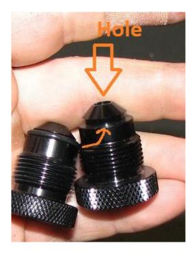
**4.3.** Fit the supplied o-ring to the black 6AN to 1/2", ensuring that it is located after the thread.
