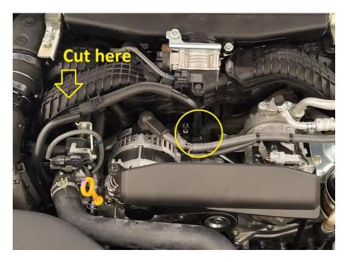
**2.17.** Where the tube meets the fitting for the engine breather tube slice the tube lightly where it is pressed onto the fitting. We recommend doing multiple light slices to prevent damaging the fitting. Once you slice through the tube, remove it.
