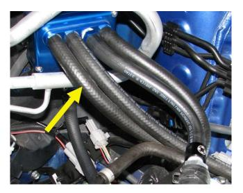
**4.6.** Remove the hose from the AOS and cut it into two pieces. One should be approximately 13 inches, and the other should be approximately 7 inches.
