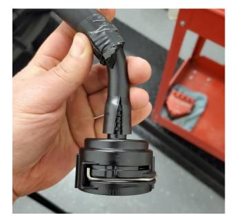
**2.17.3.** Install the fitting back on to the turbo inlet.
