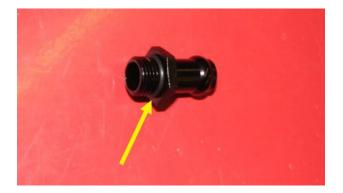
**4.4.** Then, install the black 6AN to 1/2" barb into this and torque to 8 ft-lbs. A photo of this is shown below. When installing the black 6AN to 1/2" nipple, do so with the knurled fitting already installed on the AOS.
