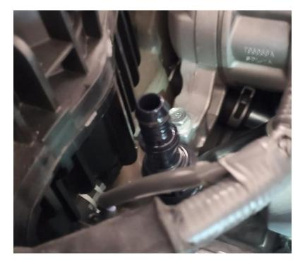
**2.17.1.** Following the other half of the tube down to the turbo inlet, you will notice there is another metal clip to release in order to remove the fitting. Take note of where the tube is routed. This is where the AOS hose will also be routed.
