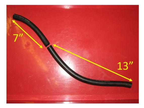
**4.7.** Install all three hoses to the car, the 7 inch section goes to the ½" adapter installed in the engine block. The 13 inch section goes to the first barbed connector on the AOS and the supplied 12 inch section goes to the drain plug on the bottom of the AOS.
