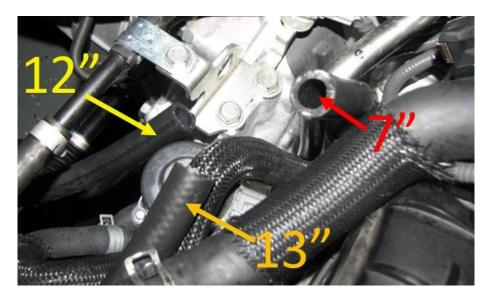
4.8. Using the supplied "Y" fitting, combine all three hoses as shown below
