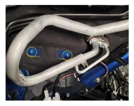
**3.7.** Next locate the throttle body coolant hose that we will need to remove. It is directly under the throttle body opening.
