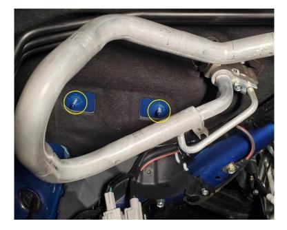
**2.6.** Remove the OEM PCV valve by first removing the large 7/8" hose, and clamps from the manifold and PCV valve itself.
