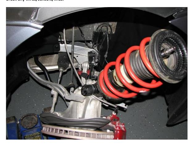
**2.11.** Remove the (4) 13mm bolts that hold the factory camber plate to the chassis.
