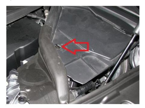
**2.5.** Remove the camber plate cover by using dikes or plastic rivet removal tool and pull upward on this to fully remove. The plastic rivets are circled in yellow.
