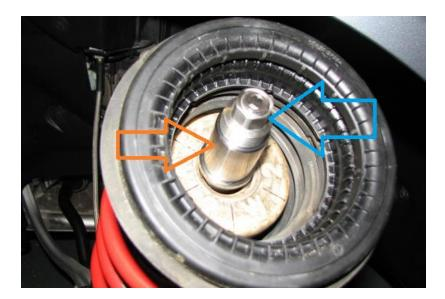
**2.13.** Install the Verus Engineering camber plate base with adjuster onto the chassis with the supplied M8 nuts and washers as shown below. The "Verus Engineering" logo should be outward on the chassis for both left and right side.
