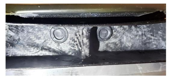
**2.19.** At this point, you may choose to reinstall the Styrofoam piece. It will require removing the middle portion as shown below. Note that it may not stay attached to the crash bar, and could fall off during the bumper install. We chose not to reinstall it.
