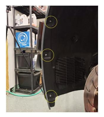
**2.4.5.** Remove the front half of the passenger side fender liner.
