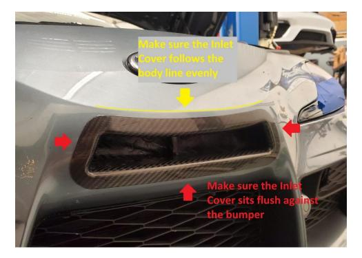
**2.17.** Once you have the Intake Duct in the ideal spot that matches with the Inlet Cover, tighten the screws for the Intake Duct. The upper screws (fine threads) should be torqued to 6 ft-lbs, and the bottom screws (coarse thread) should be tightened only a quarter turn past bottom.
