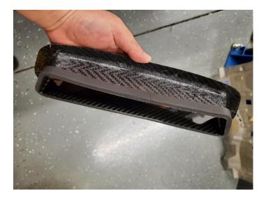
**2.23.** Apply the precut double-sided tape to the back of the Inlet Cover. The red backing should be facing you.
