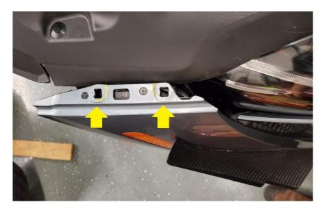
**2.4.7.** Disconnect the connectors on each side of the bumper, and unclip them from the chassis.
