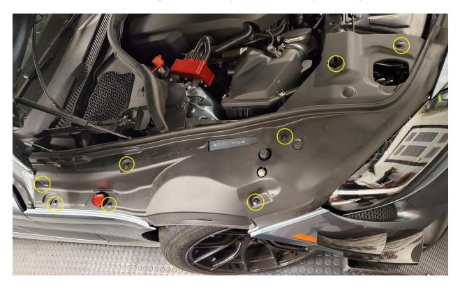
**2.10.2.** Remove the top two bolts. When removing the headlight bolts make sure to hold back the washer above the pink retainer. Again, marking the head of the bolts to ensure it is reinstalled in the same spot is a good idea.
