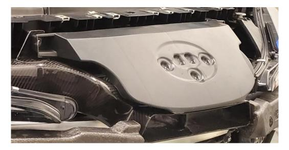
**2.18.** Install the rubber plugs into the holes in the Intake Duct.
