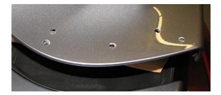
**2.9.** With the all the holes drilled, we can test fit the trunk mount. To do this, install the two studs as shown with a 3mm allen wrench. \*NOTE:\* Not all the studs can be installed and pass through the trunk at the same time, we found these two to work well.
