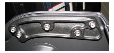
**2.19.** Install the uprights onto the trunk mount by using the M6 x 1.0 x 16mm long button head cap screws and 12mm OD washers as shown below.
