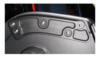
**2.18.** Using stainless washers and the stainless nyloc nuts, tighten the trunk mount and support brace to the trunk to about 6 ft-lbs. The nyloc nuts will resist backing off, so do not go over tighten these.
