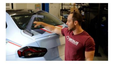
**2.20.** Now it is time to fit the wing to the car. Using a M6x22mm long SHCS, two M6x12mm OD washers, and a M6 nyloc nut, start the bolts in the front on both sides. Keep these bolts hand tight for the time being.
