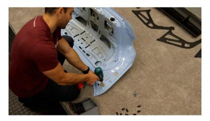
**2.10.** Flip the trunk over and grab your step bit. Open the holes on the top of the trunk to 5/8". **Note: The pink arrow indicates one of the holes that is fully opened up.**
