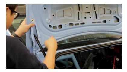
**2.18.** Install the remaining M6x25mm long SHCS with trunk mount washers in the bottom OEM mounting locations. Torque all four trunk bolts with a 5mm Allen wrench to 6 ft-lbs while ensuring the trunk is centered as well as possible. Below is a photo for referencing how everything goes together. At this point, you may reinstall the wiring harness and trunk insulator.
