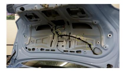
2.5. Next, we need to remove the rearmost connectors. Below is a photo of the location of the connectors and what the connector looks like removed. Note: We used a set of needle nose pliers to press in the sides of the connector to remove it. If you have stronger fingers you will not need the needle nose pliers.
