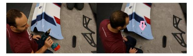
2.11. Now we need to install the standoffs as shown below. The shorter standoff (P1401A-A) is used in the rear of the trunk mount and the taller standoff (P1400A-A) is used on the front of the trunk mount. Install by hand first, and then use a 12mm wrench and torque them to 6 ft-lbs. You may also use some red Loctite here if you wish. Note: The trunk mount shown is the left-hand side (USDM driver side).
