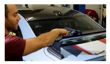
**2.21.** For AOA, below is a guideline of what we have designed and tested internally. That being said, every install and car can vary from this slightly. To ensure proper AOA, you should lay a straight edge from the front to the rear of the wing and check \*in relation to the ground plane\*.
