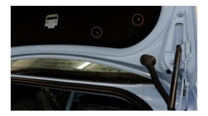
**2.4.** After the trunk insulator is removed, start removing the clips holding the wiring harness to the trunk.
