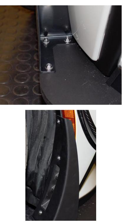
**2.11.** Tighten all the hardware with the endplate aligned with the splitter. The M4 hardware uses a 2.5mm Allen wrench while the M5 hardware is a 3mm Allen wrench.
