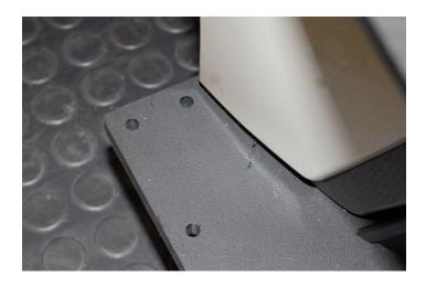
**2.10.** We can now install the endplate. Use the M4 hardware for the fender liner side, and the M5 hardware on the splitter side.
