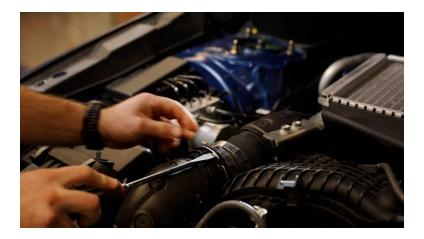
**2.5.** Fully remove the charge cooler and set aside until it is time to reinstall.
