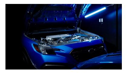
**2.3.** First, we need to remove the charge cooler. Using a 12mm socket and the driver of choice, remove the bolts securing the charge cooler.
