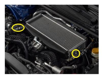
**2.4.** After the bolts are removed, use your flathead screwdriver to loosen the charge pipe clamp.
