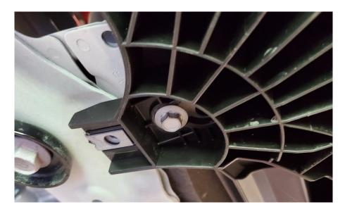
**2.8.** Finally, remove the bumper cover support brace by removing the two clips holding it in from the top.
