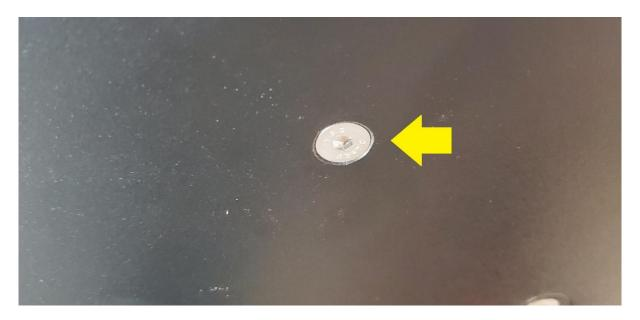
**3.13.** For the rest of the bolts, loosely install the air dam onto the splitter using the 25mm long BHCS and 18mm fender washers on the bottom side with a serrated flange nut on the top side. Only install the nuts hand tight initially. Once the splitter is on the car, we can make final adjustments for the air dam before fully tightening it down. Below is what the splitter should look like before getting installed on car.
