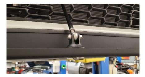
**2.37.** Use two 45mm long BHCS, fender washers, 15mm, and 5mm nylon spacers to bolt the splitter to the radiator support splash shield on both sides (the plastic cover with the metal U-nut). This is shown below.
