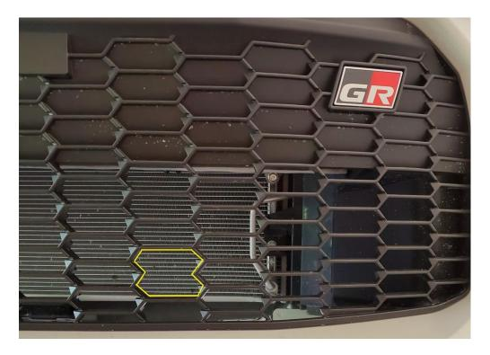
**2.23.** Bolt the splitter tie to the clevises using 25mm BHCS, 12mm washer, and M6 serrated flange nut. Do this for both sides. Torque the bolts to 6ft-lbs. The washer should be on the bolt head side.
