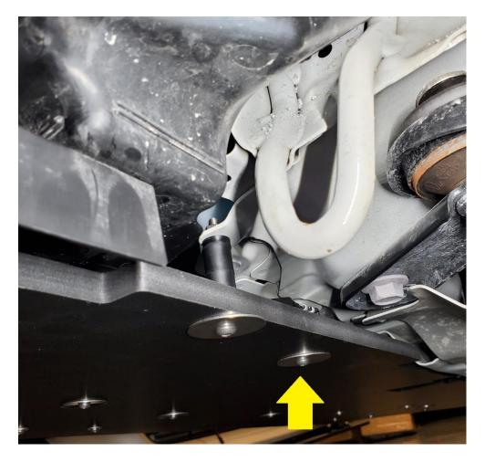
**2.38.** Then, using the 60mm BHCS, fender washer, two 15mm nylon spacers, one 5mm nylon spacer, and M6 serrated flange nut to bolt the splitter to the lower radiator support. Do this on both sides. This is shown below.
