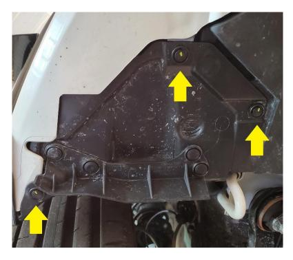
**2.6.** We are now able to remove the last push clip holding the bumper splash guard on. Pull the fender liner down and remove the clip shown on both sides. You can put the bumper splash guard aside as it will not be re-installed.
