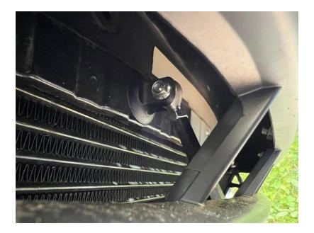
**2.32.** Re-install the radiator support splash shield with only the three bolts.
