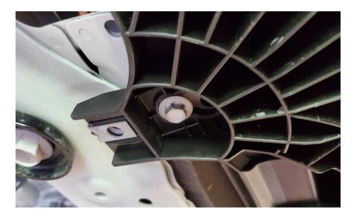
**2.33.** Next, we will begin putting the splitter up using seven 40mm BHCS, fender washers, and 5mm spacers in the holes shown below. Starting in the middle, and working your way outward is the easiest way to get this done. Do not tighten the bolts down at this time.
