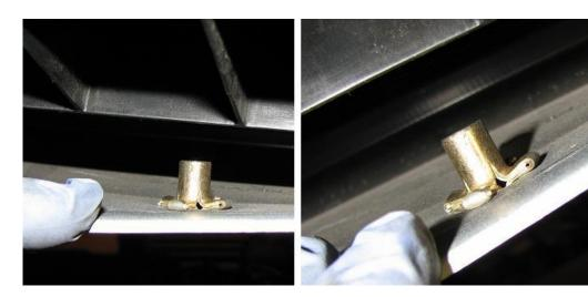
**2.13.** Re-install the bumper cover support brace back into the bumper.
