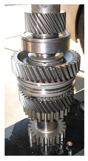
32) Install the snap ring on the end of  $6^{th}$  gear.
