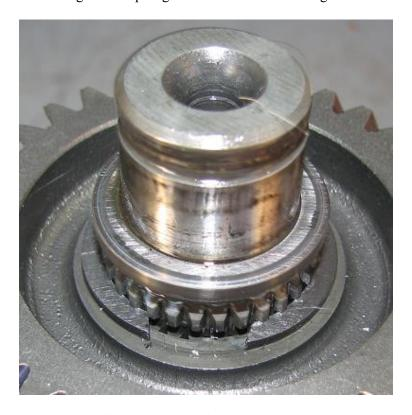
6) Remove counter drive gear from counter shaft.
