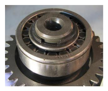
19) Remove 5<sup>th</sup> / reverse gear's clutch/shift hub assembly's snap ring via snap ring pliers.
