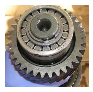
4) Using a special service tool (or 90 degree 1/8" L-brackets), press the bearing off. The fit is fairly snug.
