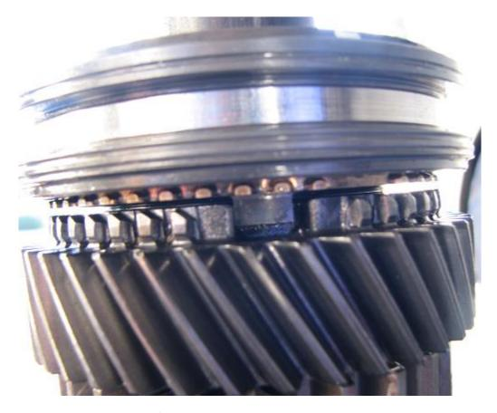
28) Below shows a picture of  $1^{st}$  gear's synchro properly installed into the shift/clutch hub assembly, you need to do this for all synchros!
