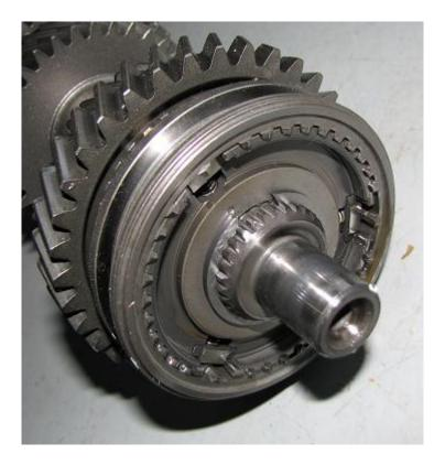
20) Press this shift/clutch hub assembly and reverse gear off as shown below. Remove the needle bearings as well.
