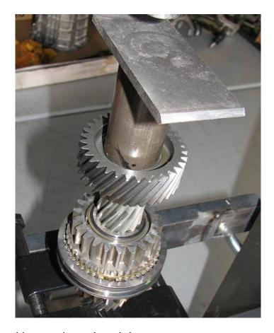
16) Install counter drive snap ring as shown below.
