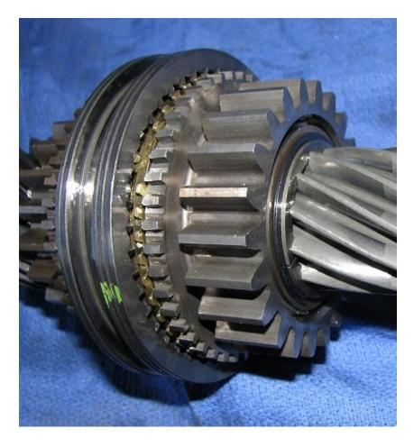
15) Press on the counter drive gear as shown below.
