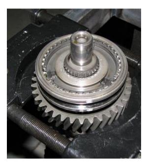
21) Remove  $6^{th}$  gear's snap ring, shown below, with two screw drivers and a hammer.
