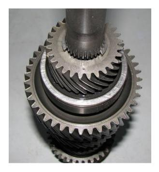
22) We remove  $6^{th}$  gear, output bearing, and  $1^{st}$  gear in one step. This requires a bit more force but all three can come off at the same time.
