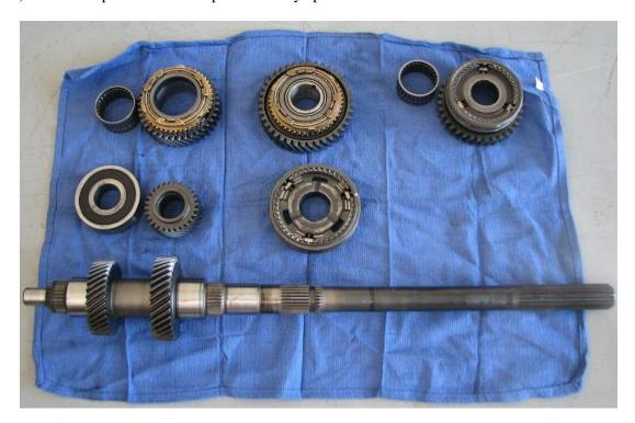
26) Time for re-install on the billet output shaft. Place  $2^{nd}$  gear's needle bearing (oiled) on the shaft, slide  $2^{nd}$  gear down on the shaft,  $2^{nd}$  gear synchro, and then the  $1^{st}/2^{nd}$  gear shift/clutch hub. This requires a long special service tool as shown below.
