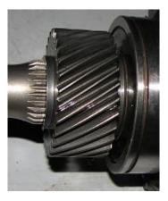
33) Reinstall reverse gear, synchro, and reverse/5<sup>th</sup> gear shift/clutch hub assembly. Install the snap ring on the end of the shift/clutch hub assembly.
