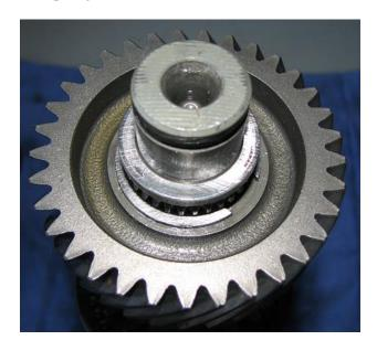
17) Install front counter gear bearing as shown below. The snap ring groove points upward.
