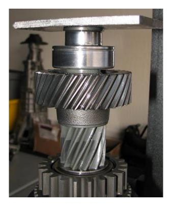
18) Install counter bearing snap ring on the freshly installed bearing. The counter shaft is finished and ready to go back in the transmission. Next up, output shaft!
