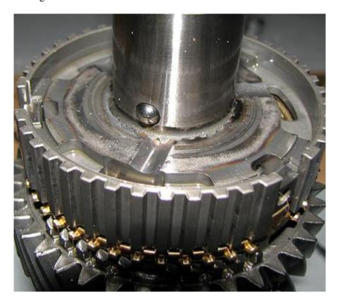
30) Install 1<sup>st</sup> gear by sliding it onto the shaft with the bearing assembly going on the inside. This will have to be spun to the correct location due to the shift restrict ball.
