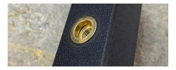
**2.24.** Once the rivet nuts are installed, thread the M6 jam nuts onto the M6 x 30mm long low-profile SHCS, and then thread the SCHS into the rivet nuts as shown below.
