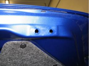
**2.21.** Now we need to install the heavy-duty rivet nuts into these holes. Use the following diagram to install the rivet nuts. **Note: The rivet nuts shown in the diagram are incorrect for this segment, but the install process is the same. The second image shows the correct rivet nuts to use here.**
