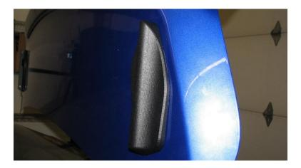
**2.14.** You can now close the trunk for the upright installation. Grab two M6 x 16mm BHCS and two 12mm OD washers and install the upright as shown below and torque to 6 ft-lbs. A 4mm Allen wrench or socket will be used here.
