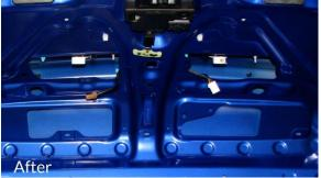
**2.5.** With the wiring loom removed from the trunk, grab your 12mm socket and ratchet, then remove the four bolts holding the trunk to the hinge arms. Having a second set of hands for this step is extremely helpful. Once removed, set the trunk down on a soft and flat surface with the bottom side facing upward.
