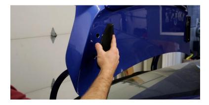
**2.13.** Once the four bolts are torqued to spec and the trunk is aligned properly, you should have something that looks like the photo below.
