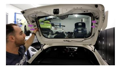
2.10. Close the rear hatch and remove the OEM wing by firmly pulling upward. Note: This can be done by yourself, but to ensure the rear hatch does not get damaged, it is always helpful to have a second set of hands with this step.
