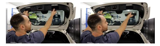
**2.7.** Once the handles are removed, grab your 10mm socket, ratchet, and ratchet extension to remove the bolts securing the trim to the hatch. There is a total of four bolts that need removed.
