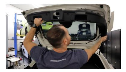
**2.9.** Remove the 10mm bolts securing the OEM wing to the rear hatch.
